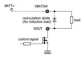
Figure 9.6: Digital output connection – open drain
