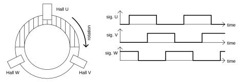
Figure 10.1: Example of UVW commutation signals
