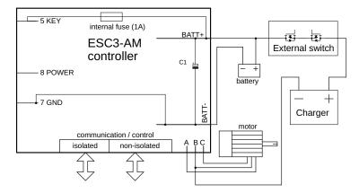
Figure 8.2: Connection of the AM controller as step-up charger
