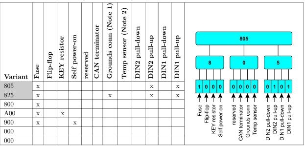
Note 1: When selected, CANGND and GND connected together - galvanic isolation is not present
