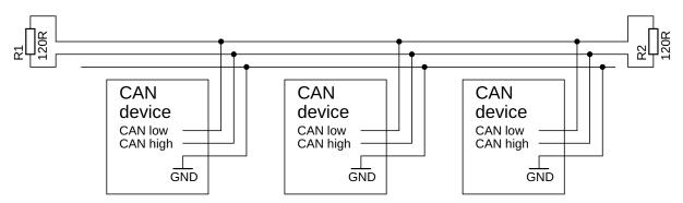
Figure 9.3: Connection of CAN Bus
