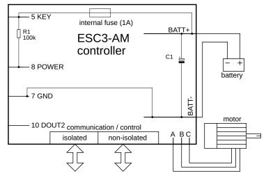
Figure 8.3: Constant on powering scheme
