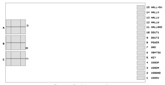
Figure 11.1: Board pinout – top side
