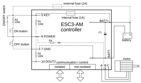
Figure 8.1: AM controller powering scheme
