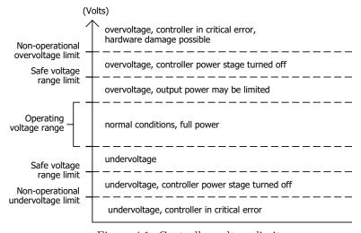
Figure 4.1: Controller voltage limits
