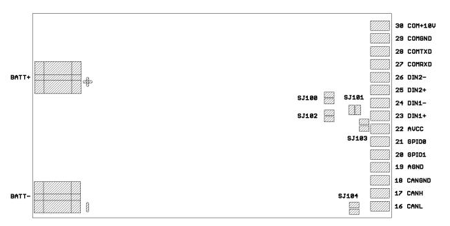
Figure 11.2: Board pinout – bottom side
