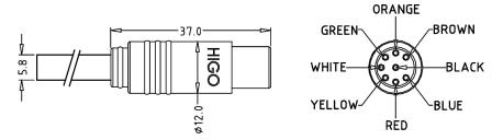
Figure 11.3: Combined wiring connector - Higo Z812AM P
