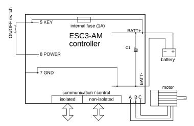
Figure 8.4: ON/OFF switch powering scheme
