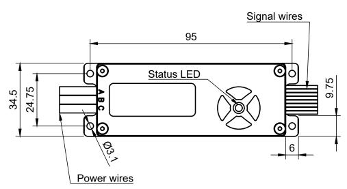
Figure 5.1: Aluminium housing for AM controller
