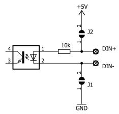
Figure 9.4: Digital input solder jumpers
