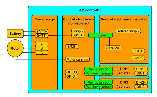
Figure 9.2: Block schematic of galvanic isolation
