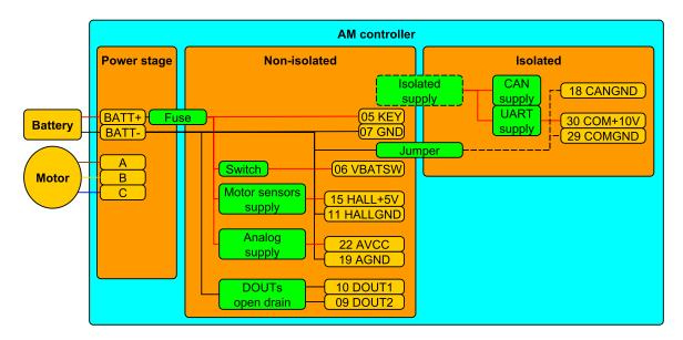
Figure 9.1: Block schematic of controller power supplies
