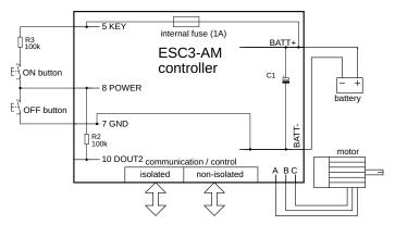
Figure 8.5: Two buttons powering scheme
