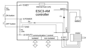
Figure 8.6: Two buttons powering scheme
