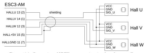
Figure 10.2: Connection of UVW commutation signal to the controller
