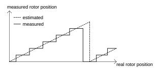
Figure 10.3: Rotor position estimation from UVW commutation signal
